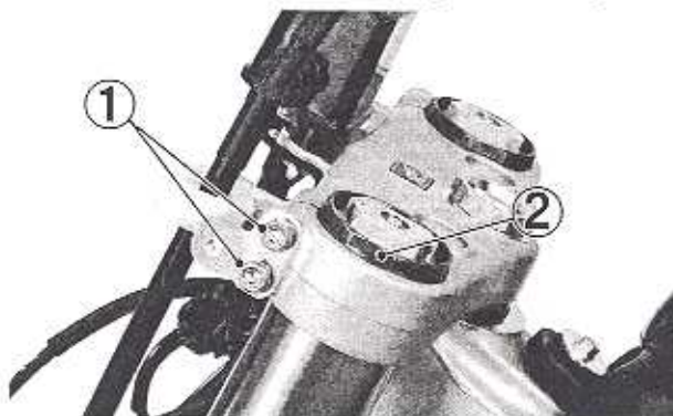
(1) UPPER PINCH BOLTS (2) FORK DAMPER
